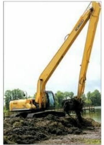
An excavator on Thursday compresses weeds and muck collected from Alligator Lake. The weeds and muck were later loaded into a dump truck and removed.
